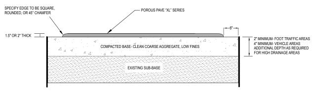
The base preparation under Porous Pave is very important. The porosity and effectiveness of Porous Pave to allow storm water to infiltrate into the ground is based on the porosity of the base and the substrate below the base. Areas of heavy soil will require thicker base to increase the holding capacity of water or may require installation of drain tile to carry excess water away.
